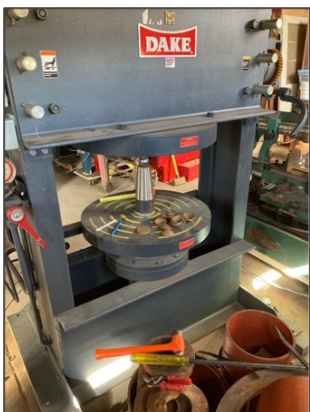
(150-ton Mechanical Press used to make Hank's head armor)
