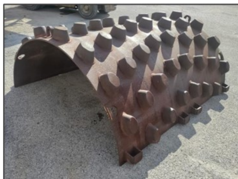
(Sheepsfoot roller used for the body)
